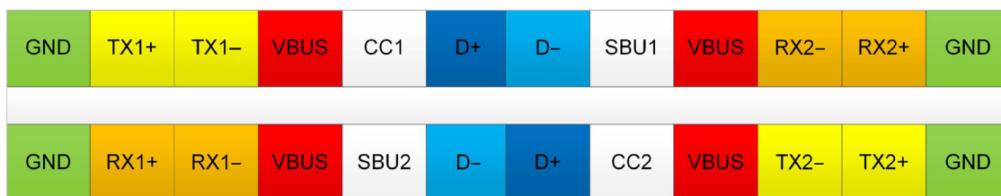
Figure 13. Type-C receptacle pinout.
